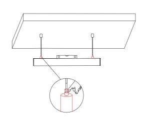
Press and hold the gripper of the lower part of the suspension to fix the aircraft cable in place.
